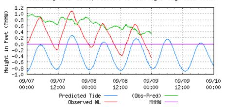
Last Observed Sample: 09/08/2017 23:54 (EDT). Data relative to MHHW Observed: -0.46 ft. Predicted: -0.80 ft. Residual: 0.34 ft. Historical Maximum Water Level: Nov 23 1988, 3.41 ft. Next High Tide: 09/09/2017 06:07 (EDT), 0.16 ft.
