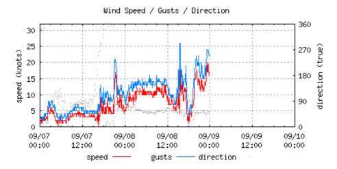
Last Observed Sample: 09/08/2017 23:48 (EDT) Wind Speed: 16 knots Gusts: 22 knots Direction: 48° T
